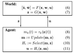
The trackers (8) provide active, time-varying assertions directly grounded in the sensor stream. Equation (9) refers to the update of the agent's knowledge representation, based on its prior state and sensor input.<sup>1</sup>
