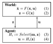
Equation (1) describes how the robot's state changes as a function of its current state and the motor vector. The function F represents the physics of the world and the robot's body, including all the complexities of motor performance,
