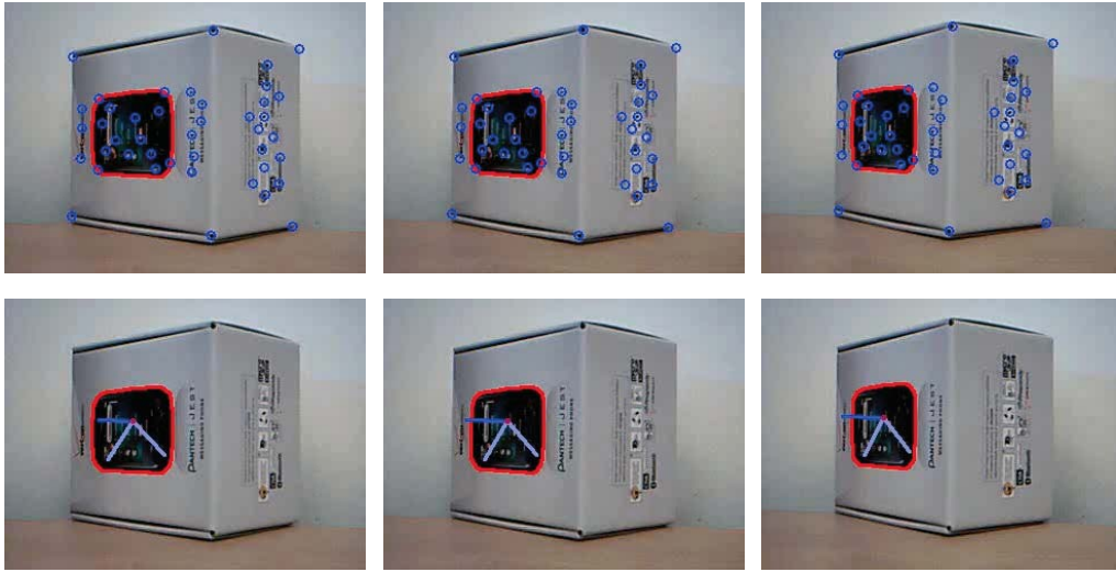
Figure 6.4: Planar region tracking and pose estimation (best viewed in color). The image sequence is captured from a commonly available webcam. Top row: tracked planar region feature and point features, bottom row: estimated normals for the planar region feature. The normals are shown in the component space (see text for details), where x-axis and y-axis (in light blue color) are on the same plane as the planar region, and z-axis (in dark blue color) is along the region normal.
