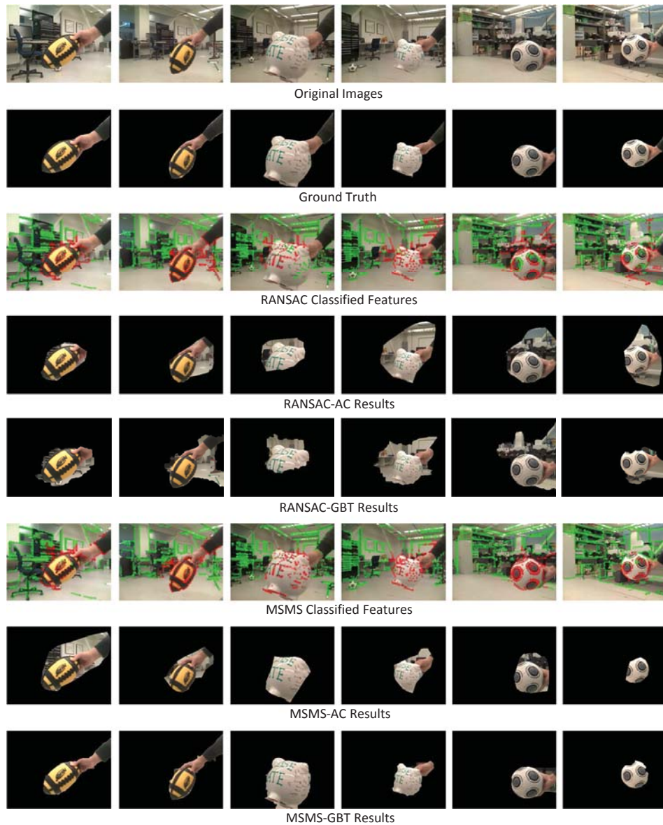
Figure 5.9: Detection results for the FM case (camera on a mobile robot). The rows show the original images, ground truth, classified sparse features by RANSAC (background in green and foreground in red), segmentation results by RANSAC-AC, segmentation results by RANSAC-GBT, classified sparse features by MSMS, segmentation results by MSMS-AC, and segmentation results by MSMS-GBT, respectively (best viewed in pdf).
