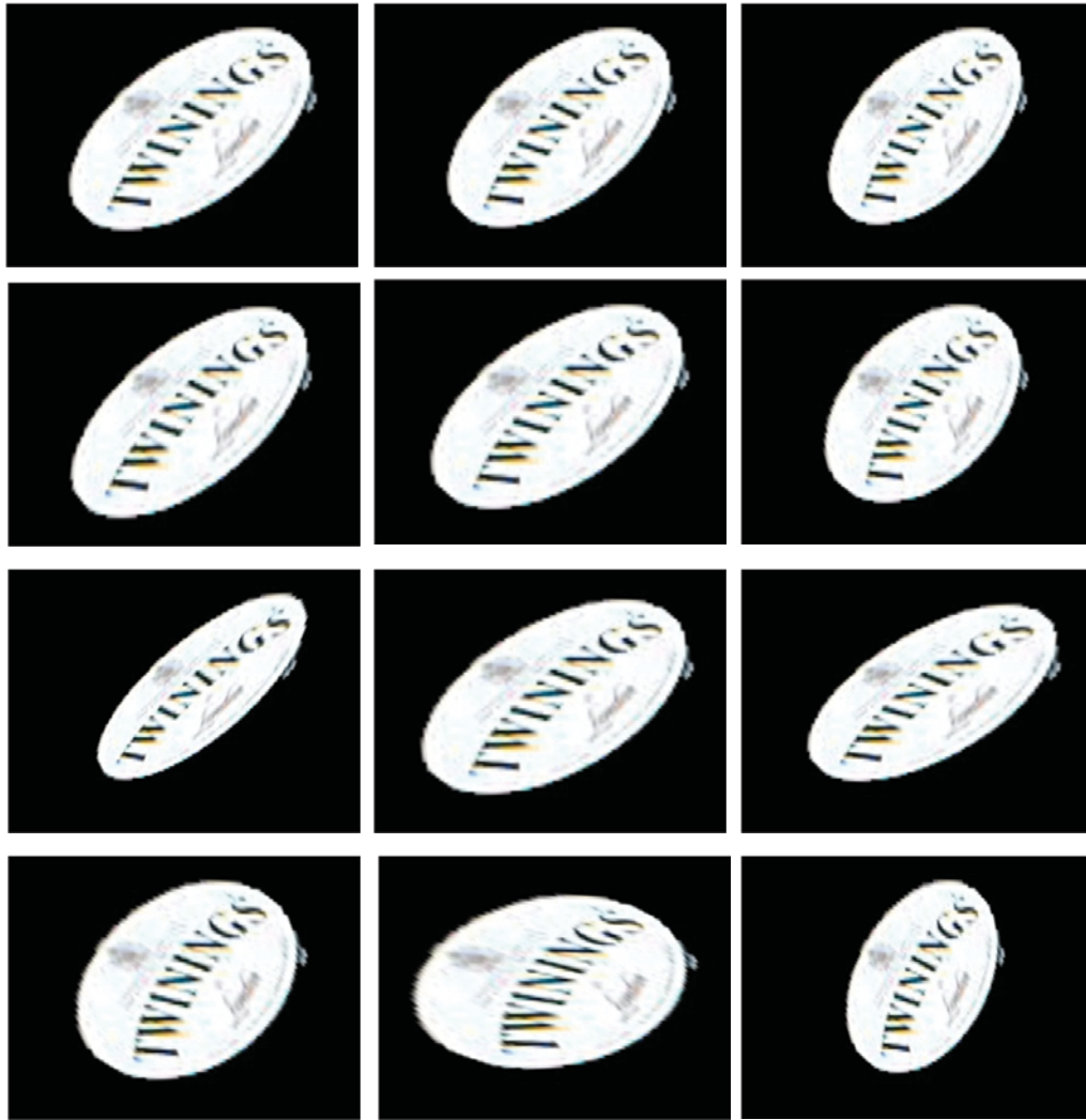
Figure 6.9: Normal views under different normal samples. Each normal view corresponds to the view of the planar component under a sampled normal of the component. The last image shows the normal view for the best normal estimate.
