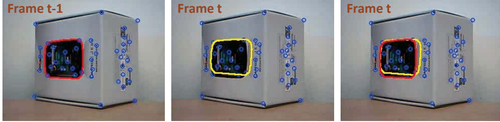
Figure 6.2: Planar region feature tracking scheme (best viewed in color). The left image shows the tracked planar region feature (red contour) and point features in frame t - 1 . The point features are tracked in frame t in the middle image using the KLT method [Shi and Tomasi, 1994], and the boundary of the planar region feature is predicted in frame t as the yellow contour using the point feature correspondences between the two frames. Then the location of the planar region feature is refined in frame t by dense pixel alignment, shown as a new red contour in the right image. Note that in our work the sparse feature tracking step is taken only between two adjacent frames, but we have intentionally enlarged the frame interval and tracking errors in this figure to clearly show the tracking scheme.
