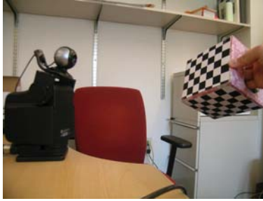
Figure 3.4: A robot looking at a checker box. A box is moving around in front of the robot, which has a webcam mounted on a pan tilt unit.
