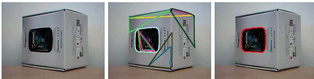
Figure 6.1: Planar region feature detection (best viewed in color). Left: input image, middle: a set of planar region feature candidates in different colors, right: the best planar region feature (red contour) used for camera pose recovery.
