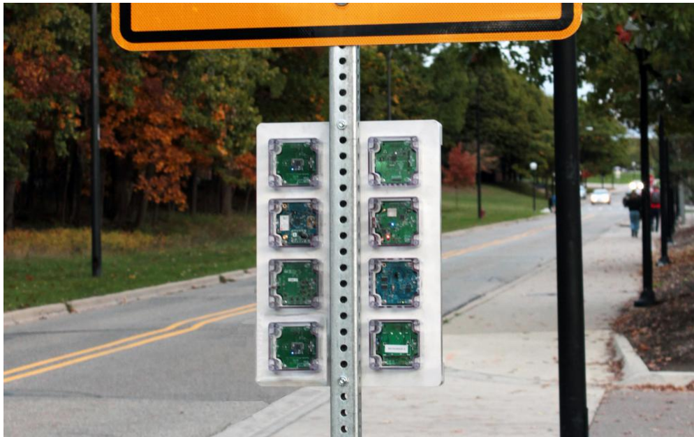
Figure 2.1: The Signpost platform easily mounts to existing street sign posts, harvests from an integrated 0.1mm solar panel, and provides tenant sensor modules with power, communications, processing, storage, time, and location. Signpost is open source, with all hardware and software available online.
