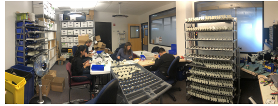
Figure 6: The PowerWatch assembly line. Over the course of four weeks, 10 undergraduates worked 110 person-hours to assemble 295 PowerWatch sensors. They were responsible for assembling the plug; screwing together the enclosure; attaching the circuit board; connecting the battery, antenna, SIM card and SD card; and provisioning the device with base firmware. They worked from team created assembly manuals and training materials.
